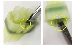
To disconnect the 6 pin connector from the unit you may need a small flat blade screw driver to release the tab holding it into the unit. The pictures to the left show the tab
