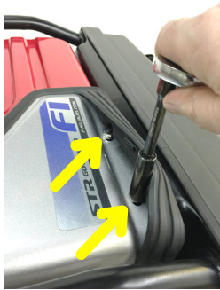
1a-2 /3 Pull back rubber gasket and remove 2 #10mm nuts then pull up and remove corner cover.
