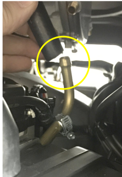
1b-1/2 Remove propane fuel tube clamp then separate propane fuel line from propane injector just above air box. Install supplied stopper into end of brass fuel injector twisting to make sure it seals hole in end.
