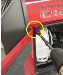
2d-6/7 Re-install door and 2 right side bolts - all 10mm bolts, then push up gasket into place.
