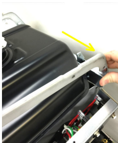
1e-4/5/6 Remove gas tank by gently prying up and away on the frame until the side rail slips free at front top edge. Take side rail out to lift out tank then lift up on tank. Then gently push front back into place.
