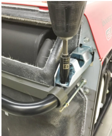
2e-3/4/5 Re-install rear handle with 4 12mm bolts then re-install exhaust shield with 4 10mm bolts then slide in front handle and secure with 4 12mm bolts.
