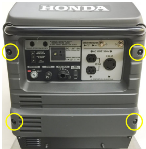
1a-3/4 Remove front shell by removing 4 corner 10mm cap nuts then remove screw from inside of fuel lever and pull out fuel lever with round label behind it. DO NOT TURN ON FUEL as a precaution.
