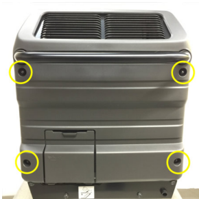
1a-6 Remove rear shell by removing 4 corner 10mm cap nuts then pulling off.
