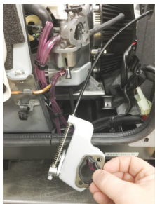
1d-1 /2 Remove choke lever assembly from carburetor by pulling entire carburetor and choke forward.
