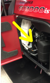
2f-4/5/6/7/8 For all states except California place Emissions label over existing EPA/CARB label on side of engine (inside door near spark plug). For California units place Emissions label next to existing EPA/CARB label. Apply medium size Propane label on top, Genconnex label on the REAR handle and small labels on sides as shown.
