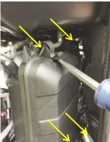
1c-1/2/3 Remove air cleaner box by first opening box and removing air cleaner element, then disconnect vent tube then remove qty 2 10mm nuts and 1 10mm bolt.
