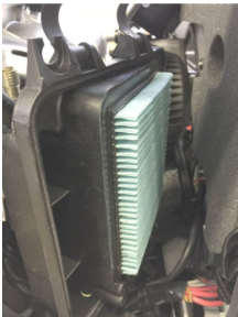
2b-5/6 Re-install Air cleaner element then snap all 4 air cleaner box clips into place and push on vent tube.
