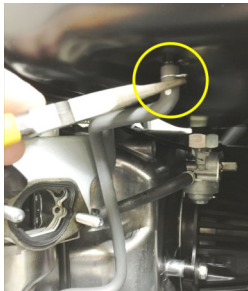
1c-4/5 Disconnect gas tank vent tube and gas line to carburetor from underside of gas tank AND from carburetor.
