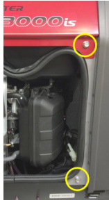
2d-6/7 Re-install door and 2 right side bolts - all 10mm bolts, then push up gasket into place.
