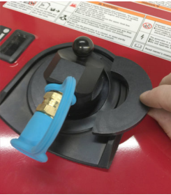
2e-1/2 Install supplied 2 clamp halves on top of unit then tighten 2 clamp bottom 5/32" socket head bolts on underside. USE CAUTION- BEWARE OF SHARP EDGES ON SHEET METAL FRAME
