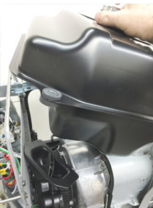
1e-4/5/6 Remove gas tank by gently prying up and away on the frame until the side rail slips free at front top edge. Take side rail out to lift out tank then lift up on tank. Then gently push front back into place.
