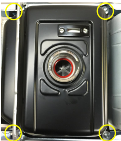
1e-3 Remove qty 4 10mm bolts and flat washers holding tank in place from top and save for later.
