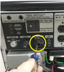
1a-3/4 Remove front shell by removing 4 corner 10mm cap nuts then remove screw from inside of fuel lever and pull out fuel lever with round label behind it. DO NOT TURN ON FUEL as a precaution.
