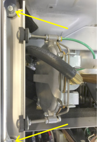
2c-1 Install gas module and secure with 2 10mm removed bolts/washers from earlier step 1d-3.
