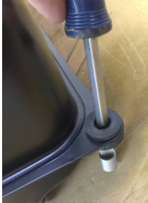
2a-3/4 Remove shock mounts from gas tank and Install 2 shock isolators onto new fuel module rail with the thickest part down.
