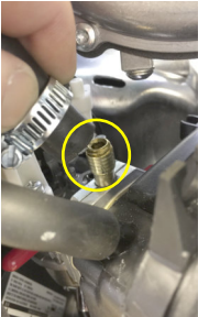
2d-1 Install new fuel line from regulator onto carburetor adapter inlet after installing correct fuel orifice (propane or nat gas)
