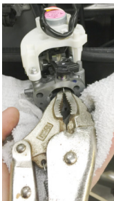
1d-4 Remove press-in choke plate with pliers then remove choke lever by pulling up and out.
