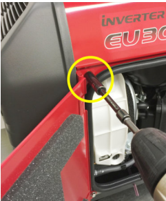
1a-1/2 Remove side access door top bolt only and pull door up and off. Remove qty 2 10mm right side bolts next.
