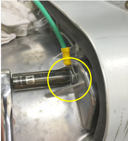
2c-2 Secure ground strap from gas module to outer frame bolt.
