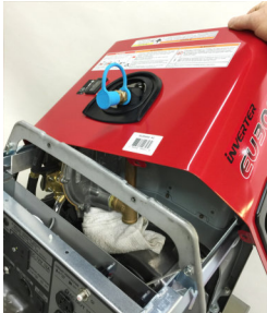
2c-4/5/6 Reposition top gasket so facing forward, then re-install pull handle assembly then pull up on gas module and tilt front edge of lid down to install cover over gas module.
