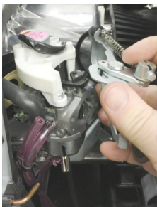
1d-1 /2 Remove choke lever assembly from carburetor by pulling entire carburetor and choke forward.
