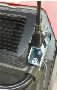
1b-1/2/3 Remove exhaust guard qty 4 10mm bolts then remove handles from front and back by removing qty 4 each 12mm bolts each.
