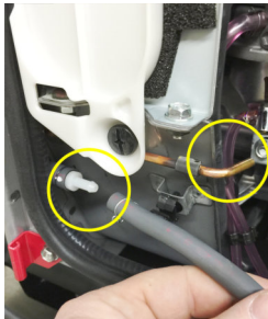
1c-6 remove two evap hoses.
