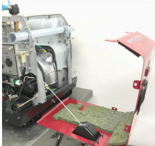
2c-4/5/6 Reposition top gasket so facing forward, then re-install pull handle assembly then pull up on gas module and tilt front edge of lid down to install cover over gas module.
