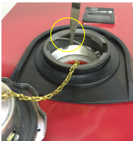
1e-1/2 Remove gas cap with needle nose pliers then lift off cover to side. Remove qty 3 10mm nuts holding pull handle unit to side and pull through. DO NOT UNTIE handle on outside from rope pull cord.
