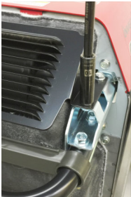
2e-3/4/5 Re-install rear handle with 4 12mm bolts then re-install exhaust shield with 4 10mm bolts then slide in front handle and secure with 4 12mm bolts.
