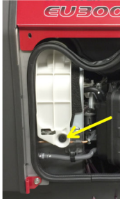
2f-3 Remove spark plug cover, gap new supplied plug to 0.020 and install.
