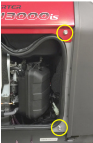
1a-1/2 Remove side access door top bolt only and pull door up and off. Remove qty 2 10mm right side bolts next.
