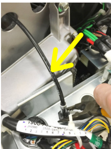
1d-5 Remove choke cable from front box and body.
