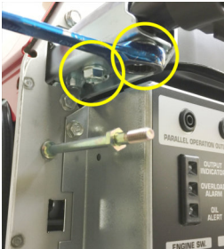
2e-3/4/5 Re-install rear handle with 4 12mm bolts then re-install exhaust shield with 4 10mm bolts then slide in front handle and secure with 4 12mm bolts.
