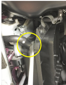
1c-1/2/3 Remove air cleaner box by first opening box and removing air cleaner element, then disconnect vent tube then remove qty 2 10mm nuts and 1 10mm bolt.
