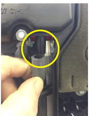
2d-1/2/3 Push fuel line all the way onto brass injector, then install air filter element, air filter cover, and then re-install crankcase vent tube.
