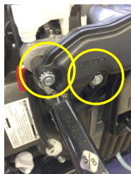
2c-4/5/6 Place air cleaner 8mm bolt through air cleaner body and add three supplied washers on backside. Hold onto washer and slide air cleaner onto upper two carburetor studs. Gently tighten 8mm bolt, then install and tighten two supplied 3/8" flange nuts to hold carburetor and injector assembly (you may need to hold 4" bolt from turning by gently pressing on side of exposed threads with finger while tightening nut).
