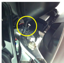
1b-1 Remove fuel line clamp at bottom of gasoline tank AFTER FULLY DRAINING GASOLINE!
