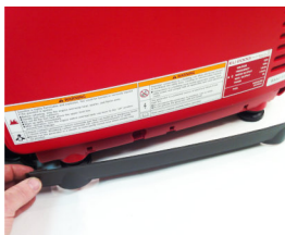
2f-7 Re-install trim (snap in place), then install back plastic cover.
