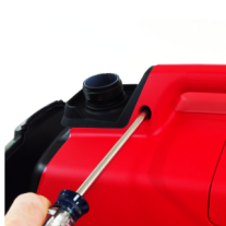
1a-7/8 Remove two handle screws.
