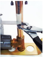
2a-1 Temporarily remove air purge knob & shaft.
