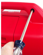
2f-1/2/3/4-install side skins by first installing 'wood' screw above pull starter then install top two screws starting with back end screw.
