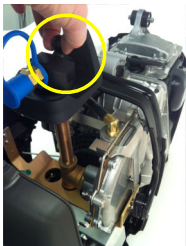
2a-3 Test air purge knob to make sure lever engages spring button and returns into seated position without binding.
