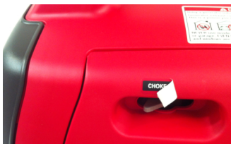
1a-1 Remove choke label (Propane does not use choke).
