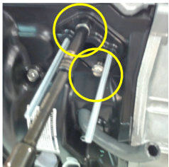
2b-1/2 Insert new long screws then re-attach block to engine.
