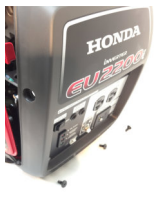
1a-4/5 Unscrew and tilt out front bezel (4 screws).
