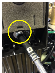
2c-4/5/6 Place air cleaner 8mm bolt through air cleaner body and add three supplied washers on backside. Hold onto washer and slide air cleaner onto upper two carburetor studs. Gently tighten 8mm bolt, then install and tighten two supplied 3/8" flange nuts to hold carburetor and injector assembly (you may need to hold 4" bolt from turning by gently pressing on side of exposed threads with finger while tightening nut).
