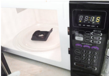
2a-2/3/4 Remove Honda gas boot from old gas tank and install over inlet (heat with hot water or carefully microwave for 15 seconds to softens it) CAUTION - RUBBER WILL BE HOT WEAR SUITABLE GLOVES.
