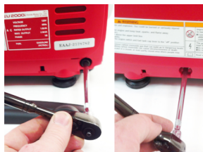
2f-5/6 install bottom two 10mm long hex bolts starting with back bolt.
