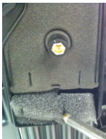
1c-1/2/3/4/5/6 Remove air cleaner unit by first removing outer cover then one inner 8mm hex bolt, vent tube, then two outer 8mm hex nuts then slide off air cleaner assembly. discard 2 8mm nuts
