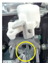
1d-1/2/3 Remove pressed-in choke plate by pulling outward with pliers (use force), then turn handle full right then pulling up. Discard choke plate, handle and felt washer.
