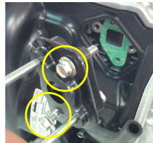
1g-1/2/3 Remove two 8mm long bolts holding carburetor to engine by removing two shorter 8mm flange bolts. Save short bolts, but discard 2 long bolts.
