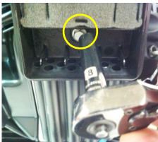
1c-1/2/3/4/5/6 Remove air cleaner unit by first removing outer cover then one inner 8mm hex bolt, vent tube, then two outer 8mm hex nuts then slide off air cleaner assembly. discard 2 8mm nuts
