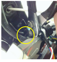
1f-1/2/3/4/5 Remove and discard gas pump & line to carburetor by moving away clamp first. Then pull off tube going to engine vent below carburetor remove gas lines from plastic holders (leave bracket in place for new fuel line). Then remove clamp on pump hose & clamp going down to the on/off switch. Lastly remove two screws holding pump to frame and discard screws and pump assembly.
