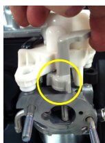
1d-1/2/3 Remove pressed-in choke plate by pulling outward with pliers (use force), then turn handle full right then pulling up. Discard choke plate, handle and felt washer.
