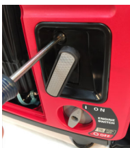
2f-1/2/3/4-install side skins by first installing 'wood' screw above pull starter then install top two screws starting with back end screw.
