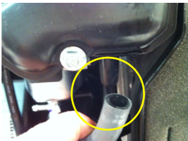
1c-1/2/3/4/5/6 Remove air cleaner unit by first removing outer cover then one inner 8mm hex bolt, vent tube, then two outer 8mm hex nuts then slide off air cleaner assembly. discard 2 8mm nuts
