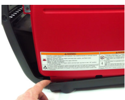
1a-9 Remove lower trim (this side only) by prying off with finger or flat blade screw driver.
