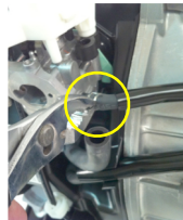
1f-1/2/3/4/5 Remove and discard gas pump & line to carburetor by moving away clamp first. Then pull off tube going to engine vent below carburetor remove gas lines from plastic holders (leave bracket in place for new fuel line). Then remove clamp on pump hose & clamp going down to the on/off switch. Lastly remove two screws holding pump to frame and discard screws and pump assembly.
