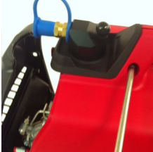
2f-1/2/3/4-install side skins by first installing 'wood' screw above pull starter then install top two screws starting with back end screw.
