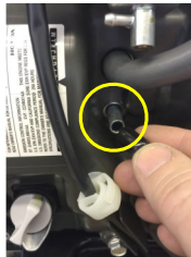
2b-5/6/7 Install red caps on carburetor inlets, small black cap inside choke lever hole, and large black cap over crankcase port.
