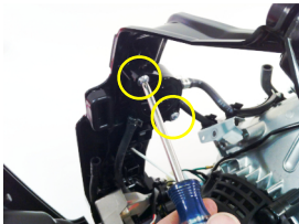
1f-1/2/3/4/5 Remove and discard gas pump & line to carburetor by moving away clamp first. Then pull off tube going to engine vent below carburetor remove gas lines from plastic holders (leave bracket in place for new fuel line). Then remove clamp on pump hose & clamp going down to the on/off switch. Lastly remove two screws holding pump to frame and discard screws and pump assembly.
