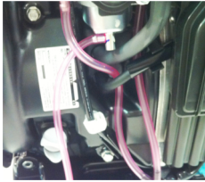
1b-3/4 Remove fuel drain & vent tubes (3 tubes) and discard.
