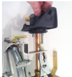
2a-5/6/5 Re-install air purge knob & shaft then adjust for 1/8" (+/- .1/16") clearance between spring button and lever. DANGER - MAKE SURE THERE IS A GAP or you will have propane leaking when you connect to your BBQ tank!
