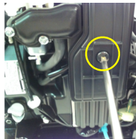
1c-1/2/3/4/5/6 Remove air cleaner unit by first removing outer cover then one inner 8mm hex bolt, vent tube, then two outer 8mm hex nuts then slide off air cleaner assembly. discard 2 8mm nuts
