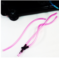
1b-3/4 Remove fuel drain & vent tubes (3 tubes) and discard.
