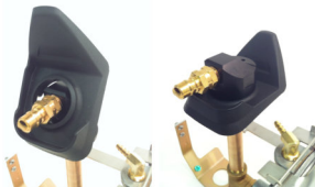
2a-2/3/4 Remove Honda gas boot from old gas tank and install over inlet (heat with hot water or carefully microwave for 15 seconds to softens it) CAUTION - RUBBER WILL BE HOT WEAR SUITABLE GLOVES.
