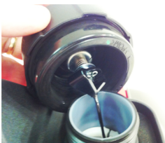
1a-3 Remove gas cap by removing cotter snap pin.
