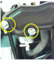
1c-1/2/3/4/5/6 Remove air cleaner unit by first removing outer cover then one inner 8mm hex bolt, vent tube, then two outer 8mm hex nuts then slide off air cleaner assembly. discard 2 8mm nuts
