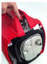
2f-1/2/3/4-install side skins by first installing 'wood' screw above pull starter then install top two screws starting with back end screw.
