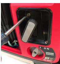
1a-12 Remove screw near pull handle.
