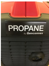
2g-1/2/3 Attach "Genconnex start" label on door next to pull start and the small "Propane" label below it, the LARGE "Propane" Label on opposite side and a small "Propane" label on the back. Place Emissions label over existing EPA label on engine frame near oil dip stick.
