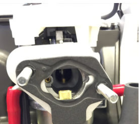
2c-1/2 Slide on the new gasket then slide on the fuel nozzle assembly then slide on the old gasket.
