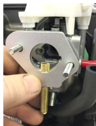
2c-1/2 Slide on the new gasket then slide on the fuel nozzle assembly then slide on the old gasket.
