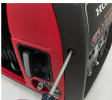
1a-4/5 Unscrew and tilt out front bezel (4 screws).
