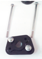
1g-1/2/3 Remove two 8mm long bolts holding carburetor to engine by removing two shorter 8mm flange bolts. Save short bolts, but discard 2 long bolts.
