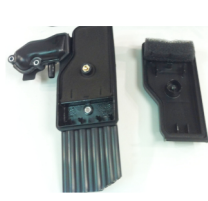
1c-1/2/3/4/5/6 Remove air cleaner unit by first removing outer cover then one inner 8mm hex bolt, vent tube, then two outer 8mm hex nuts then slide off air cleaner assembly. discard 2 8mm nuts
