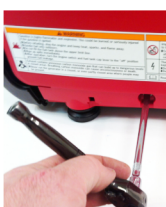
1a-10/11 Remove lower skins bolts (2 10mm bolts).
