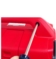
1a-7/8 Remove two handle screws.
