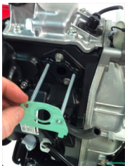
2b-3/4 Re-install gasket then slide carburetor back on Make sure servo wire is not tight on left side.
