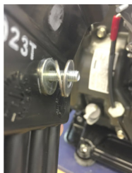
2c-4/5/6 Place air cleaner 8mm bolt through air cleaner body and add three supplied washers on backside. Hold onto washer and slide air cleaner onto upper two carburetor studs. Gently tighten 8mm bolt, then install and tighten two supplied 3/8" flange nuts to hold carburetor and injector assembly (you may need to hold 4" bolt from turning by gently pressing on side of exposed threads with finger while tightening nut).
