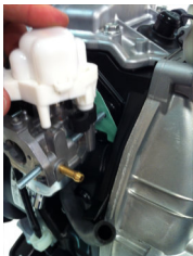
2b-3/4 Re-install gasket then slide carburetor back on Make sure servo wire is not tight on left side.
