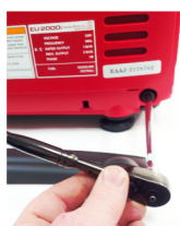
1a-10/11 Remove lower skins bolts (2 10mm bolts).
