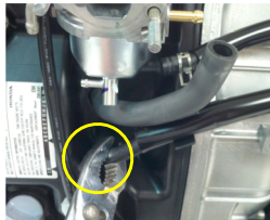
1f-1/2/3/4/5 Remove and discard gas pump & line to carburetor by moving away clamp first. Then pull off tube going to engine vent below carburetor remove gas lines from plastic holders (leave bracket in place for new fuel line). Then remove clamp on pump hose & clamp going down to the on/off switch. Lastly remove two screws holding pump to frame and discard screws and pump assembly.
