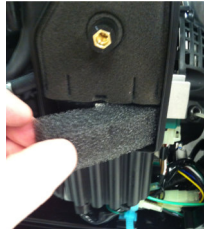
2d-1/2/3 Push fuel line all the way onto brass injector, then install air filter element, air filter cover, and then re-install crankcase vent tube.
