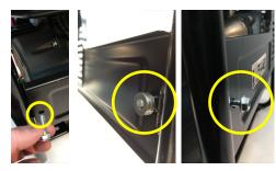
2a-2/3/4 Install supplied #10 bolt (longer than original) in it's place but only far enough to support 6 supplied washers. NOTE if you screw this bolt in too far you will not be able to perform the next step.
