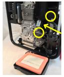
1a-3 Remove Air Filter cover and air filter, then remove lower support bracket's #12 bolt and upper #10 bolt.
