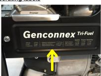
2d-2 Apply supplied rating label to back muffler guard as shown.
