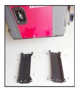
**Step 1:** Support unit on wooden blocks then remove both bottom rails with 12mm socket.
